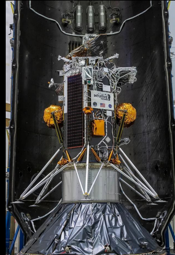
Odysseus folded up in the payload bay of the Falcon 9 before the fairings cover it Credit: SpaceX
