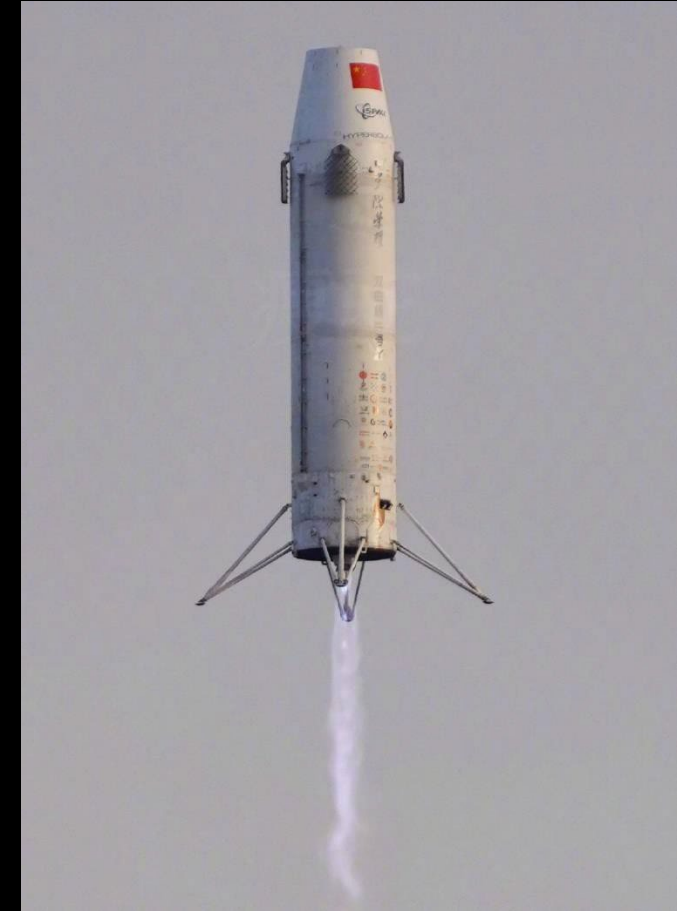
A Kuaizhou reusable prototype rocket during a short-duration launch and landing test in January 2024 Credit: KevinJamesNg
