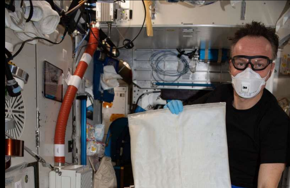
ESA astronaut Matthias Maurer changes out the bladder in the space station's Brine Processor Assembly Credit: NASA
